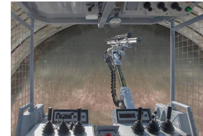
The control deck can be raised 1540 mm.
